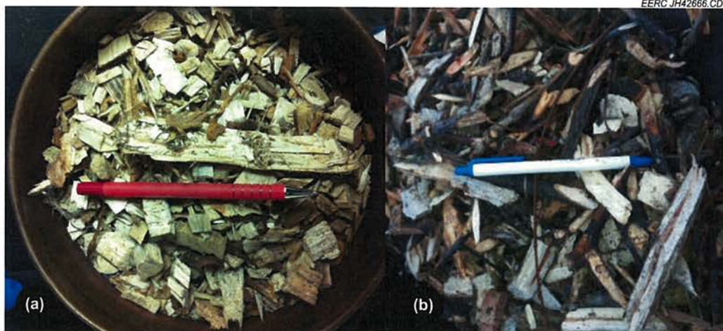
Figure 3. Biomass used in the experiments: a) chipped green poplar wood waste and b) city wood waste, primarily chipped ash.
