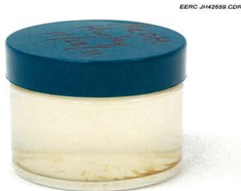
Figure 4. A jar of the liquid product several days after production showing the yellowish color and precipitate that develops in the liquid.
